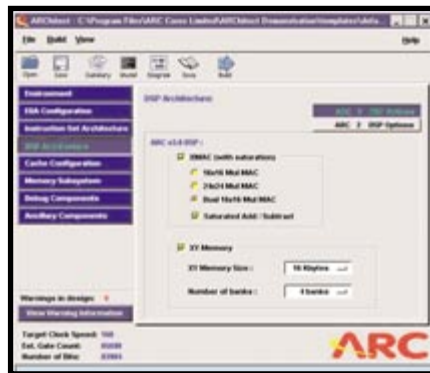
Photo 1 —ARChitect is a program that allows engineers or programmers to design their own CPU with only a few mouse clicks.
